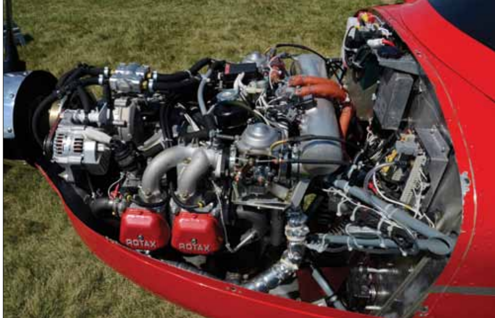
The engine compartment of the Sling 4 with the Rotax 914 turbo is a busy place. With dual carburetors and liquid cooling, the plumbing is a little more complicated than most homebuilders are used to, but the package provided by The Aircraft Factory is complete.
