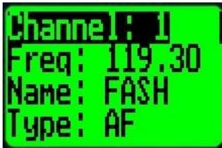
The V10 provides 100 channels for pre-programmed frequencies. Each channel contains frequency, name of the frequency (for example airport name) and type of the frequency (for example "Tower").
