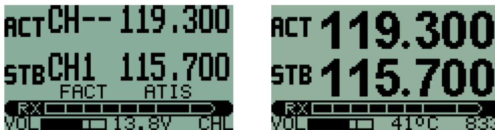
The spacing between frequencies may be in steps of 25KHz or 8.33KHz. This may be set in the Second Level Menu. A 'speed-up' function is provided for the FREQUENCY knob so that a new frequency or channel may be set up quickly and easily.
