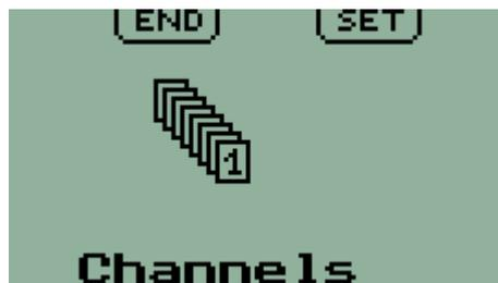
The V6 provides 99 memory channels for user programmed frequencies. Each channel has an associated frequency, 'Name' for the frequency (for example airport name or code), and 'Type' for the frequency (for example "ATIS").
