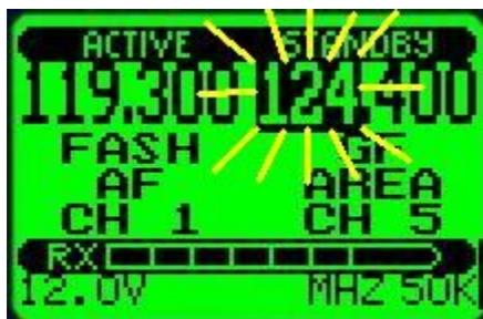
While the desired entry is flashing, you can change the number using the up and down arrow buttons.
