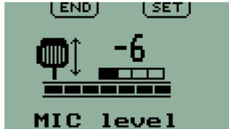
NB: For a single microphone, the level shown by the bargraph is for the Pilot microphone input ONLY. No level is shown for the passenger microphone. The adjustment affects all microphones equally.
