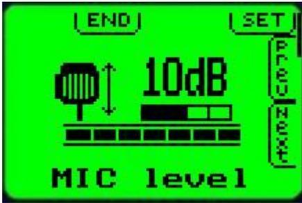
This function allows you to adjust your microphone level. A bargraph is provided so you can adjust to the correct level. The correct level is achieved if most of the time, while you are speaking normally into the microphone, the bargraph remains between about  $\frac{1}{2}$  to  $\frac{3}{4}$  of the range with excursions all the way to the right only during very loud parts of your voice or “click” sounds.
