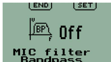
This can help reduce the effects of unwanted noise, in particular at low and high frequencies. This filter has a sharp cutoff for frequencies below 500 Hz and above 2.4KHz.
