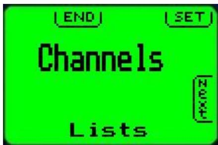
If at least one list containing at least one frequency has been uploaded to your V10 transceiver, you will be presented with a new menu entry (first level menu). This menu function allows you to select either the normal 100 channel memory to be used for channel selection or you can select from any of the uploaded frequency lists. For example the next picture shows the selection for a list called "KLAX", Los Angeles International.
