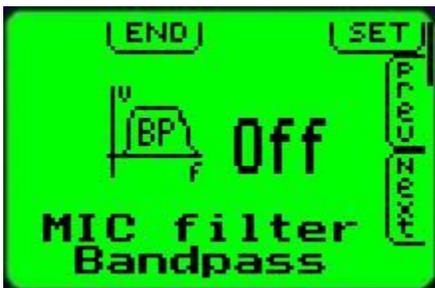
For operation with high ambient noise levels an additional voice bandpass filter can be engaged for both pilot and passenger microphone circuits.
