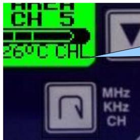
Transceiver is in channel entry mode. Pressing MHZ/KHZ/CH will allow you to change channels
