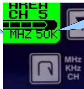
Pressing and holding the MHZ/KHZ/CH button for one second will change to 25KHZ tuning steps (8.33KHZ for European models).
