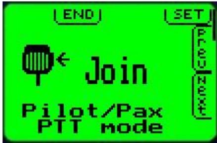
The V10 transceiver has two PTT inputs, one for the pilot circuit and one for the passenger circuit (PAX).
