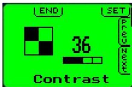
Adjust the display contrast. A value of between 30 and 40 is suitable for most environments. A lower value results in a lighter display while a higher value results in a darker display. Adjust the contrast such that dark areas are fully saturated while light areas do not show any darkening.
